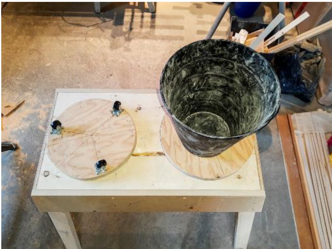
The wheels get screwed to the bottom of the wooden disks and the baskets are screwed to the top of the disks.
